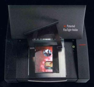
Easy to Use ► Just line up your transparent or reflective original on the built-in light table and close the magnetic FlexTight holder. Simply click your mouse and the holder is automatically fed into the scanner as your original is scanned. With an unbeatably low prep time (5 second pre-scan, and a fast final scan), productivity is boosted to an average of 15 images per hour. Since no glass plates, gel or tape are used, no clean-up is required after scanning - saving even more time.
