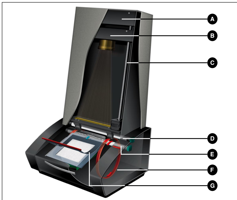
Figure 3: Cut-away view of Flextight Precision II
